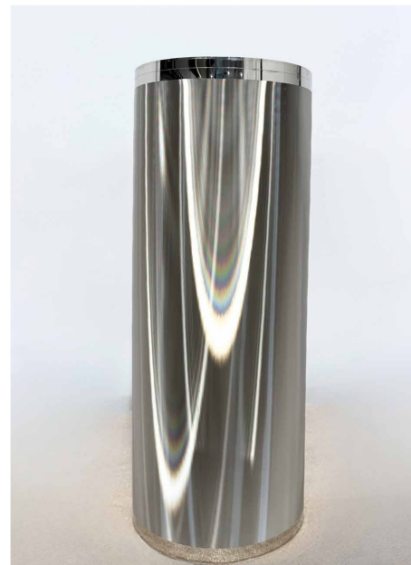
Figure 9: Laser welded sleeve during the optical inspection.
